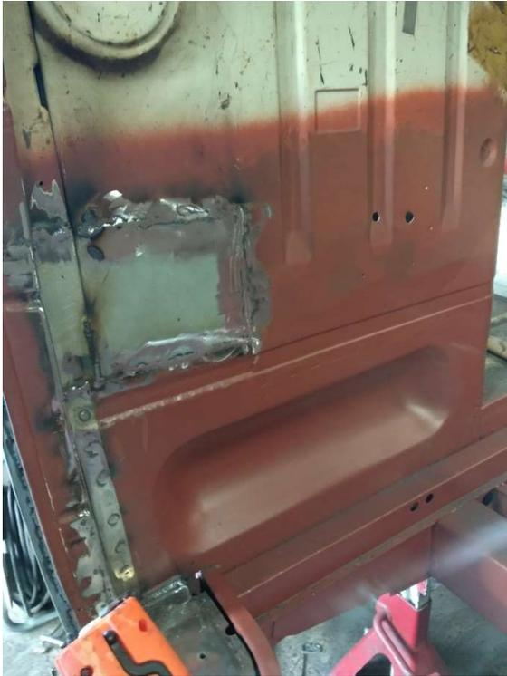
We also filled in the hole above the bulge to replace the previous rot and the top of the bulge was whacked repeatedly to make the pressing just above the bulge. It isn't perfect, but is sufficiently close that once the primer and paint are on, it should not be visible.
