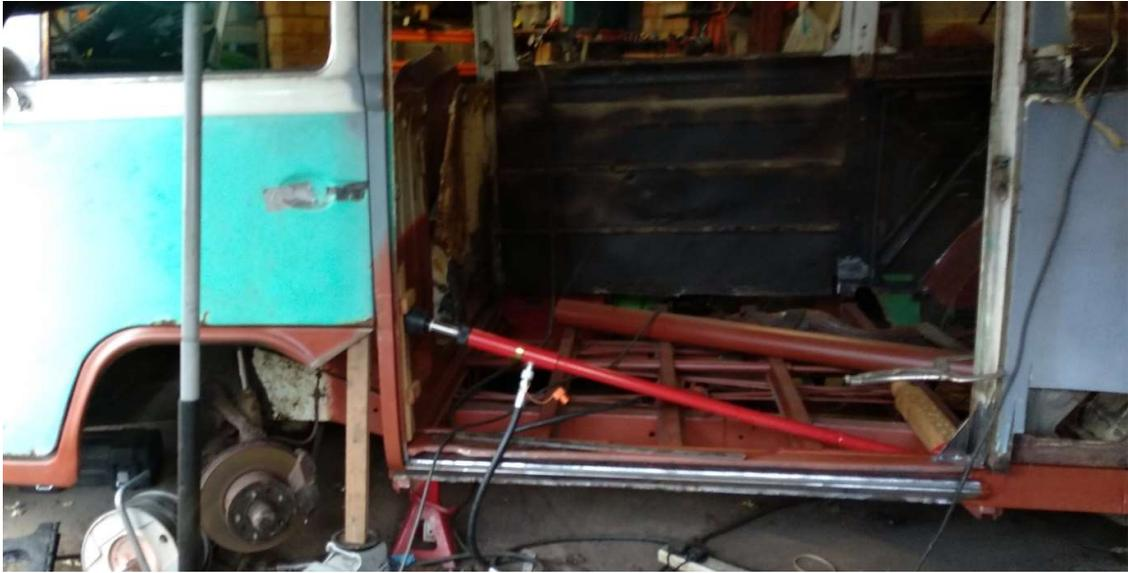
After about 4 man days, the old threshold plate, along with a new bulge, new inner and middle sill and some newly cut and fitted sheet steel are all in Eric, he is a lot stronger and it is all in the right place. 4 man days is a lot less than the 62.5 hours noted at the top, more next time. Stay dirty everyone.
