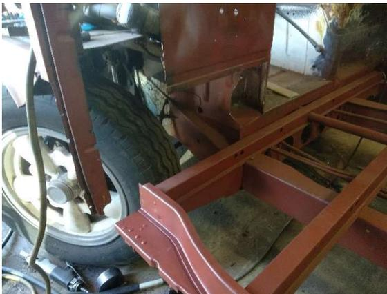
Now that all of the wrong metal was missing, including the heavy angle iron added 2 years ago for strength but in completely the wrong place, we were able to add in some good new metal in the right place. Firstly, we removed the threshold plate that you step on when entering the sliding door, we were then able to add the inner sill, then the middle sill. With those welded in place, the bulge can be fitted.
