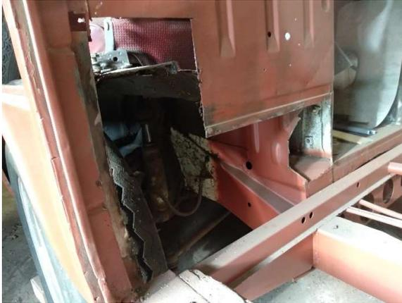
Eric's front cross member that starts this hoop runs across behind the front seats with jacking points below and SHOULD meet the edge of the B post.
