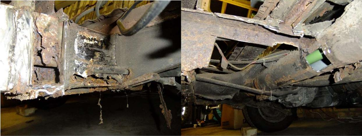
Repairing the tube is difficult as access from above is tight due to the rear panel between the wheels and welding in a confined space laid under a rotten bus is just no fun. Next job then is to remove the panel between the wheels.... All the spot welds drilled out carefully and start easing the panel away. Turns out that panel forms part of the fuel tank ledge, so a wasted hour and now need to make that good again.
