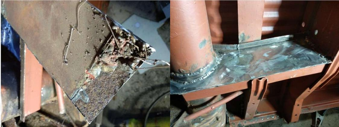
Poor welding inside the box section and new metal welded to badly corroded metal. Chopped it out and replaced it. New 2mm lightly galvanized steel sheet, cut to shape. 6mm holes drilled through it to the rest of the existing chassis box section are then plug welded thoroughly using a hot welder setting to ensure really good penetration as this is a section that needs a lot of strength!
