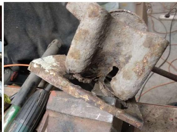
Behind the pictured circle of steel is the mounting bracket, the second picture shows that bracket from above still attached to the chassis box section. Both pieces badly holed and rotting nicely. I cut the chassis box section off the bracket and welded the bracket back together on the bench (see the shiny steel in the next photo!).
