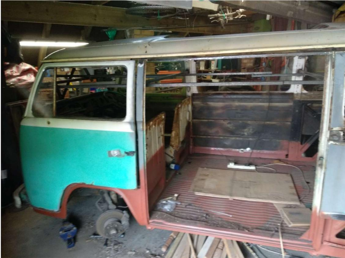
For the first time in many years, Eric has a metal roof with no rot and as you can see, further metal in the new floor as reported earlier this year. That passenger door is the one that will get a new skin in due course. With the roof in position, a few ratchet straps pulled things into place, the angle grinder neatened things up and the new roof was sitting on the front and rear temporary supports.
