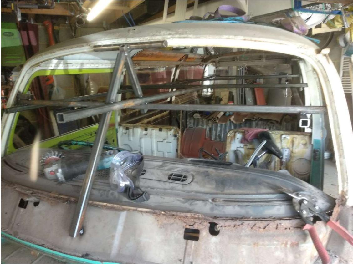
In the meantime, the steel box section had gone into Eric's interior, all welded securely to the posts to stop Eric falling apart and to give us a guide for the new roof (top middle of the above picture).
