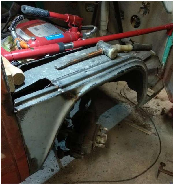
With the Porta Power stretching the door gap to the correct size and the US import door supplied with Eric's purchase making its first appearance, the wheel arch and B post were welded in place to provide strength in that area for the first time in years. Here's the view from inside – the lower 8 inches are new, fabricated inside and a Just Kampers B post outer panel on the outside.
