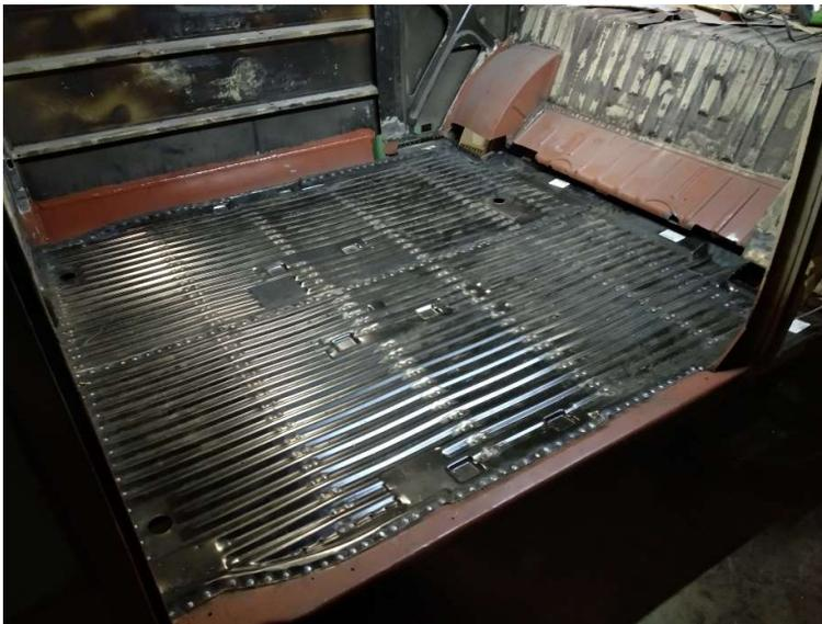
Welding took around an hour and a half of those same few hundred drilled holes and no grinding has yet happened. Given that they are all in the valleys of the corrugations, they may just get a wire wheel smoothing then some paint! As you can see, around the edges of the
