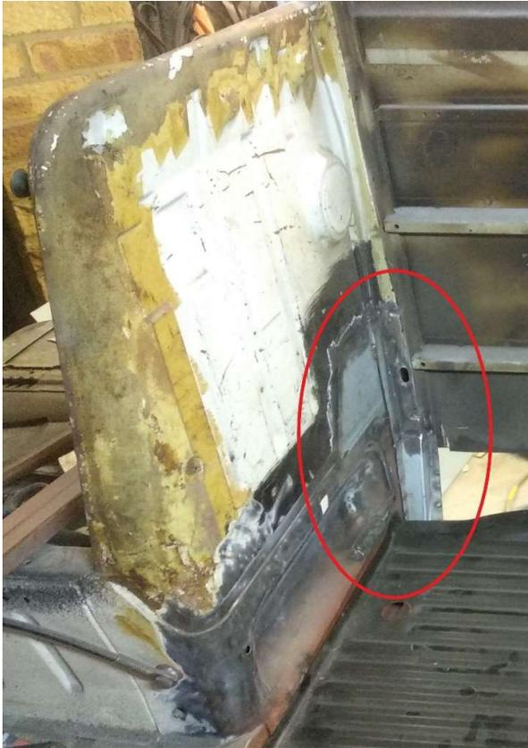
Where the floor was trial fitted, anything underneath will be hidden and received 2 brush-painted coats of oil based rust proofing primer (Rustoleum) inside the sill cavities and around the newly rebuilt B post. Anything above there will be visible inside the van and received a spray coat of Rednox anti-rust paint. Both are red!
