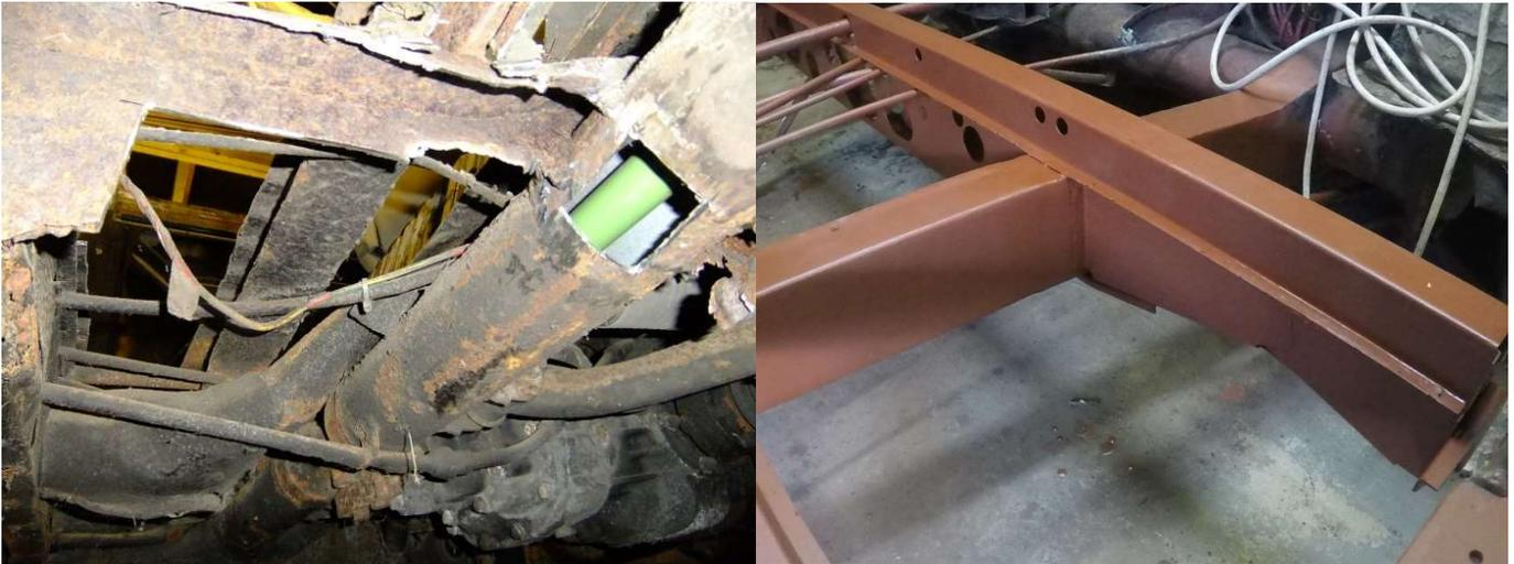
Then the B posts at the back of the driver and passenger doors and if you have them the bulkheads that sit at the back of the seats has a rail along the same line under the floor. See the picture of the rust before and the shiny new metal afterwards. All this takes a great deal of time.
