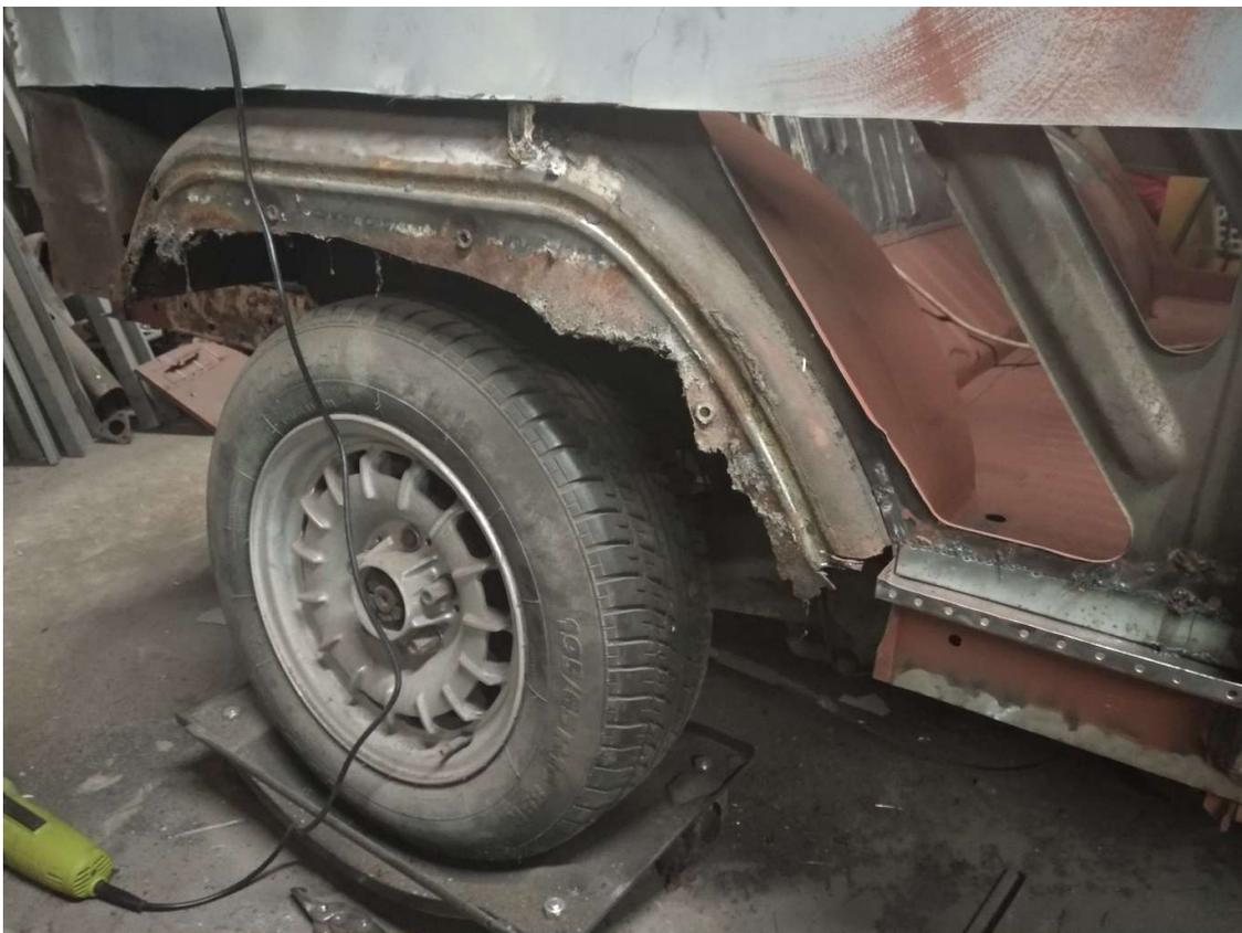
Underneath a lot of filler was a replacement outer wheel arch. That was loosely attached to another outer wheel arch that had been bent to make something approaching an inner wheel arch. That in turn was barely attached to some rust. See the above picture. This time the outer panel was trimmed slightly higher than the other side because it was about 1mm above the line of the previous outer panel. The added advantage that I can attach the new panel much easier as I will discover later. I hope.
