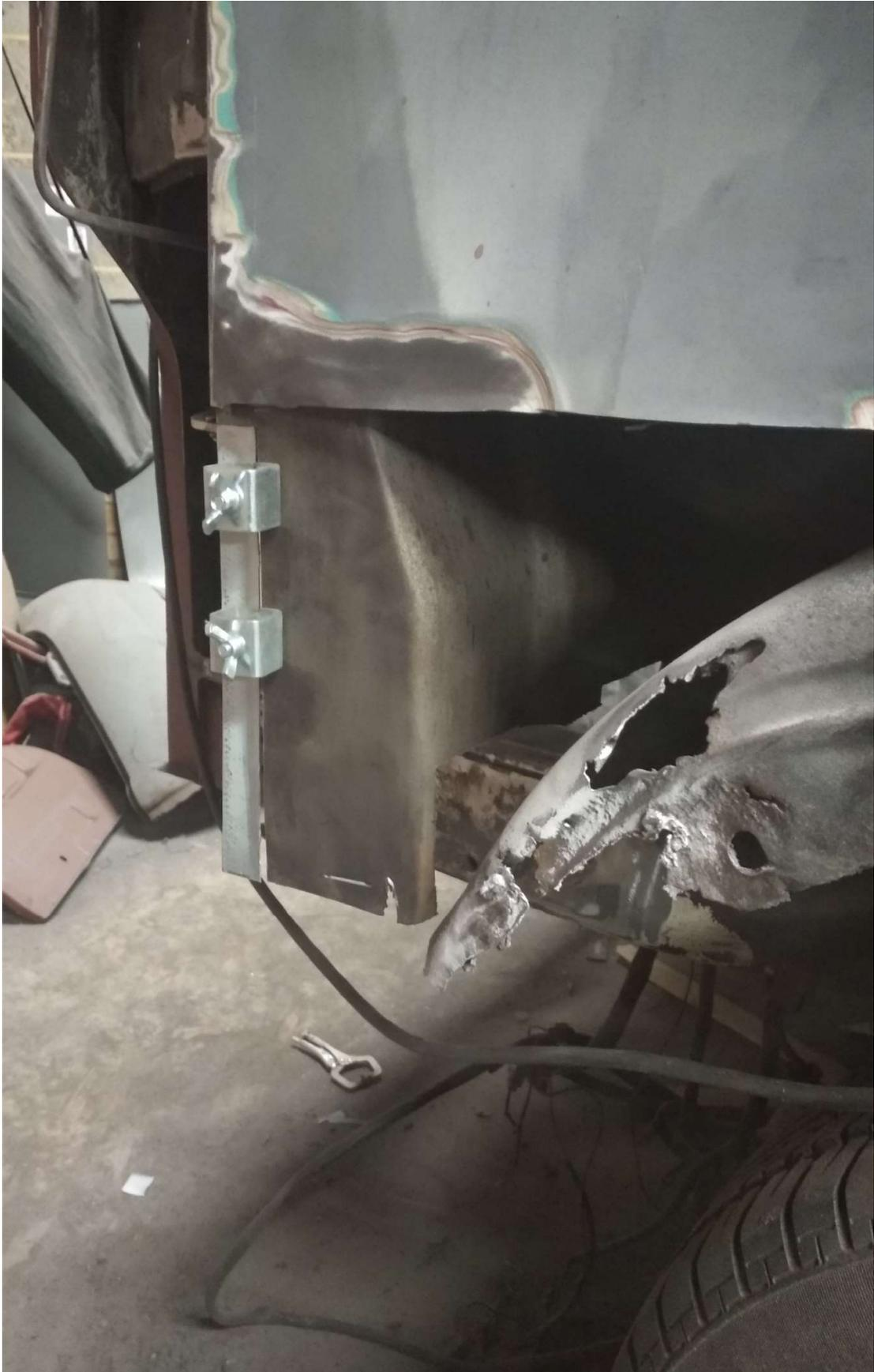
The box in the middle of the picture was missing its left edge that folds around out of shot. That edge gets the wheel arch panel spot welded to it. Then the rear corner welds to that once the battery tray has been put back in. The new piece is being held in place with my new aircraft clamps that line both pieces of metal up, hold them in place and set the gap between them all in one hit as noted previously.
