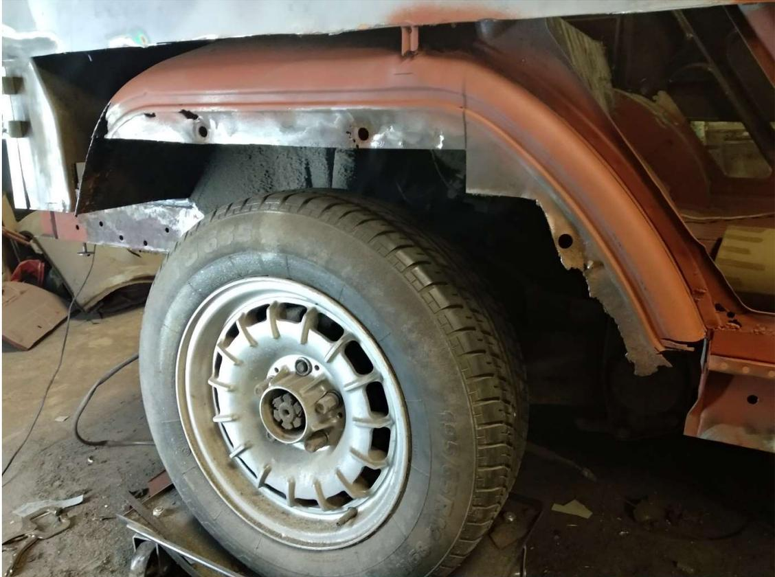
Then I used one of the outer arches suitably trimmed down to fabricate a new inner arch for the piece that I needed and clamped it in place.
